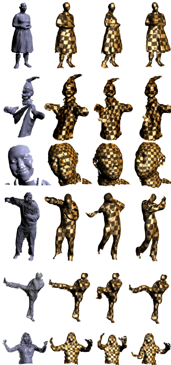
Fig. 12. Original data (left) and reconstruction with parameterization of the “Saskia”, “Puppet”, “Face”, “Abhijeet”, “Kicker” and “Woman” data sets for different poses.
