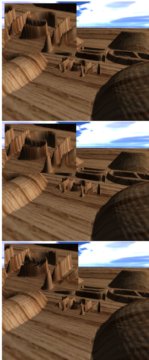
Figure 9: Rendering quality of different algorithms, renderings performed at the same frame rate. Maximum mipmaps (top), linear + binary search (center), relaxed cone stepping (bottom). The resolution of the height field is 1024^2 . The frame rate is 27 FPS (for maximum mipmaps and linear binary search). The sharp spikes are produced by antialiased font rendering into the height field. Note that relaxed CSM and linear + binary search can miss thin structures, whereas maximum mipmaps render thin structures correctly.
